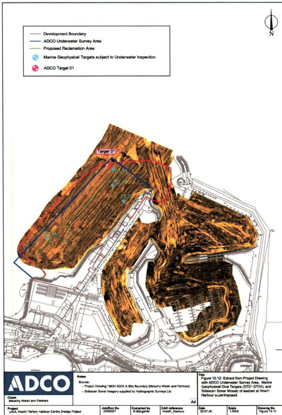
Figure 10.12: Extract from Project Drawing showing ADCO Underwater Survey Area, Marine Geophysical Survey dive targets, and side-scan sonar mosaic
