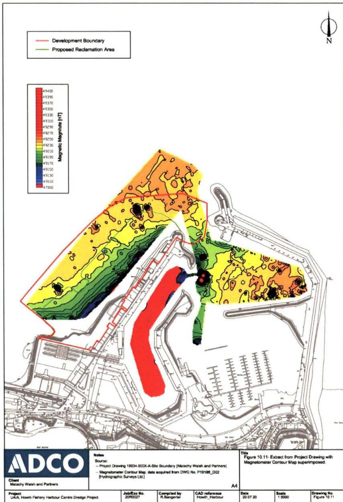
Figure 10.11: Extract from Project Drawing showing magnetometer contour map
